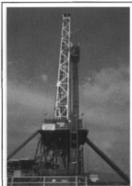
A new integrated fluids management approach and contractual model were used to successfully drill the 18,417-foot L.M. Broussard No. 1 exploratory well in the Vermillion Parish area onshore southern Louisiana. The well was drilled to total depth 45 days faster, on average, than other wells in the area, and disposable drilling wastes were reduced by 43 percent compared to the best available offset.
