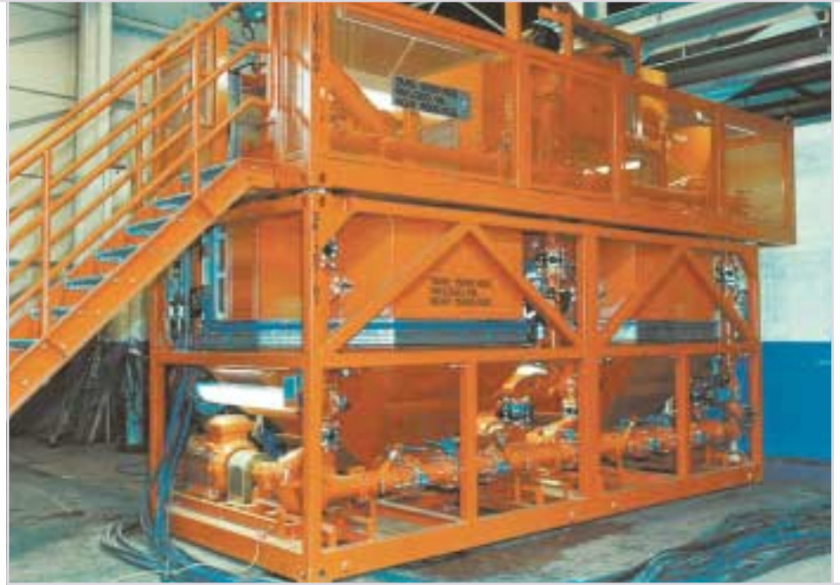
Mobile cuttings re-injection unit destined for Croatia. Its design allows transport from rig to rig and field to field.
